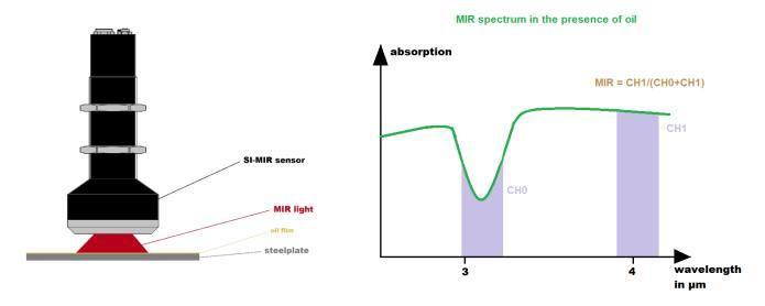
The left-hand measuring window CHO detects the extra absorption caused by the oil layer, whilst the right-hand measuring window remains largely unaffected by this.
