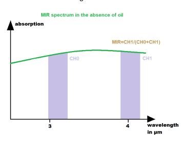
The **SPECTRO-M-10-MIR/(MIR1+MIR2)** sensor if fitted with exactly this wavelength window. A schematic depiction and initially aimed at a steel surface (without oil layer). The absorption in both wavelength
