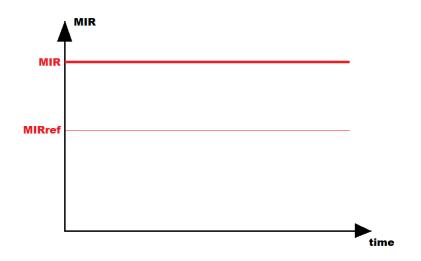
MIR=CH1/(CH0+CH1) moves upwards in the CH0 window through the additional absorption. The more intensive the absorption, i.e. the thicker the oil layer, the further removed is the MIR value from the reference value MIRref (without oil layer).
